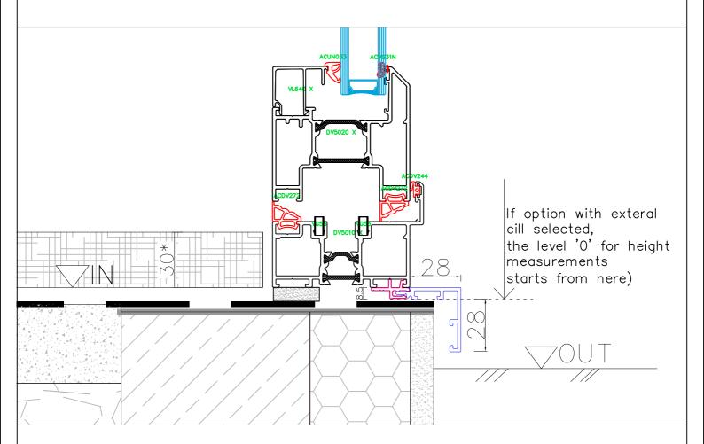
\* maximum height of the non-movable frame which can be covered by tiles, carpet, floor heating etc. is 30mm.
